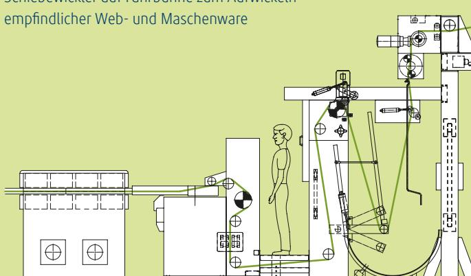
Stenter with 2-position batcher and plaiter for woven fabric or coated fabric
