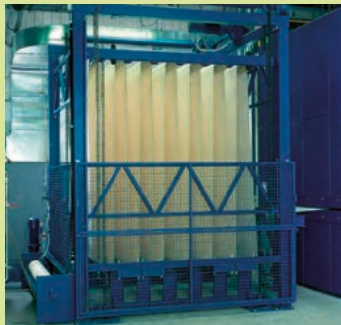
Roller-type fabric accumulator for woven fabric
