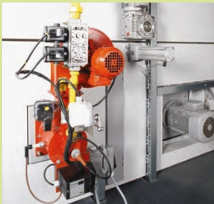
Gas burner at a stenter
