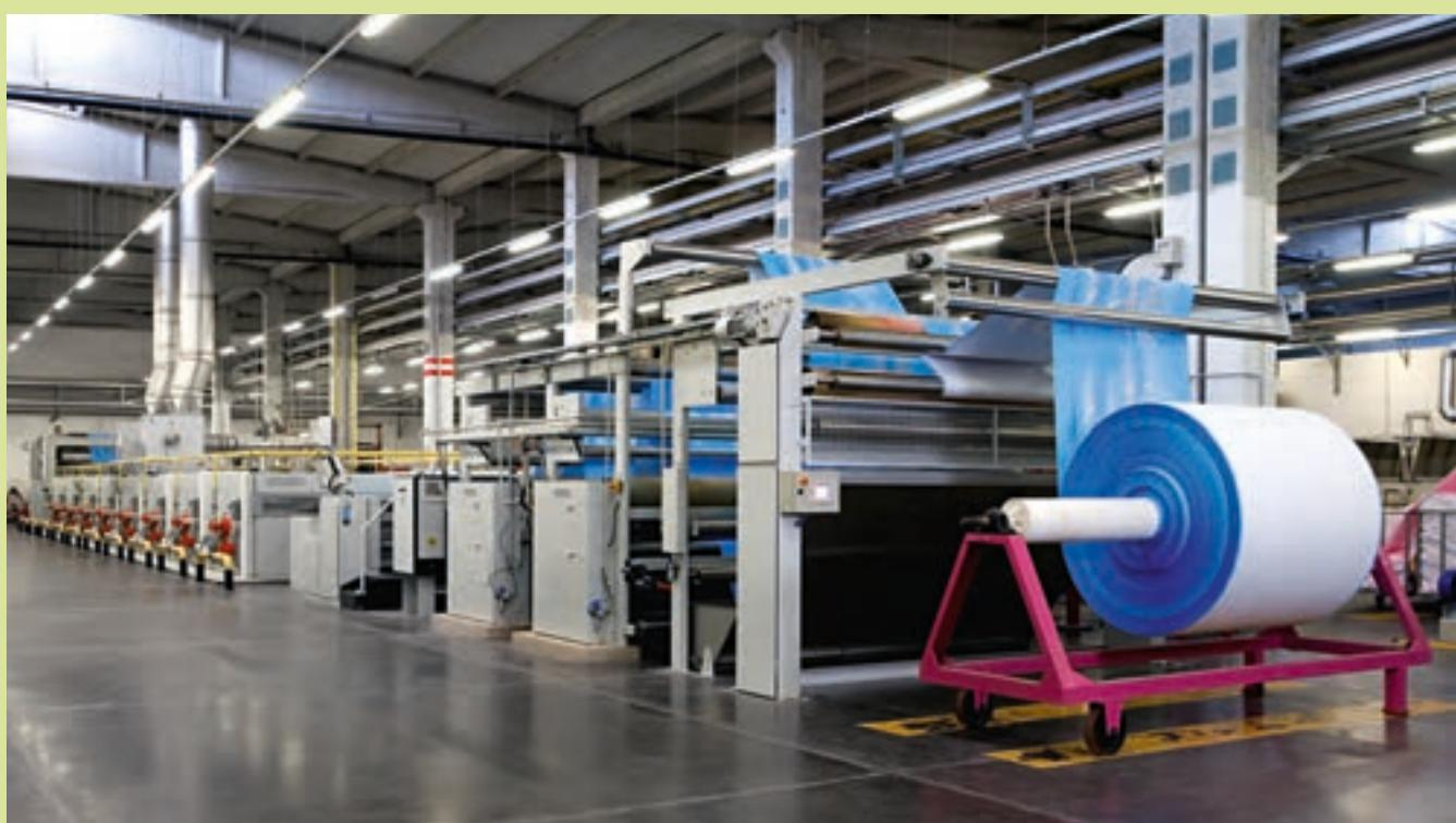
Stenter with two padders, horizontal chain and gas heating
