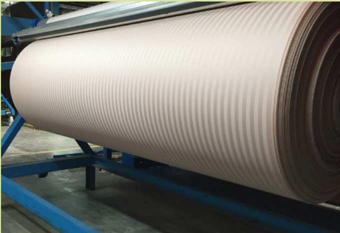
Stripe satin dyed on the BRÜCKNER POWER-COLORTHERM line
