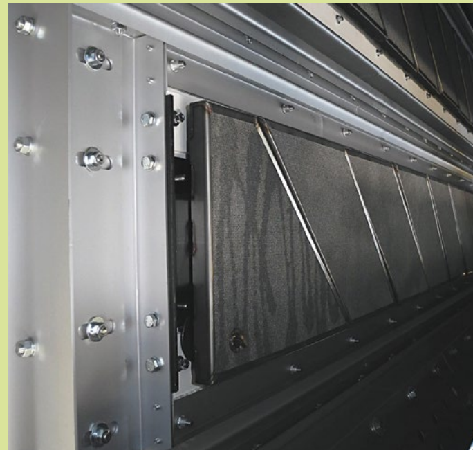
Burner elements made of special metal fibre material
