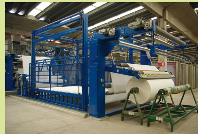
Fabric accumulator and batcher in the exit area
