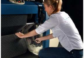
DRC30 harness frame height can easily be adjusted
