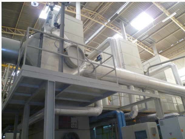
Vertical dryers : Fresh air flap, open if HE idle
