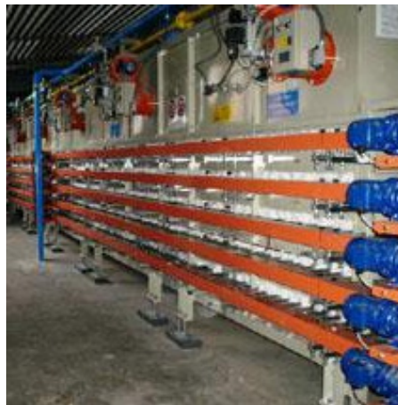
Vertical Dryer: raw tiles are dried to ~3% humidity Horizontal Multi Layer Dryer
