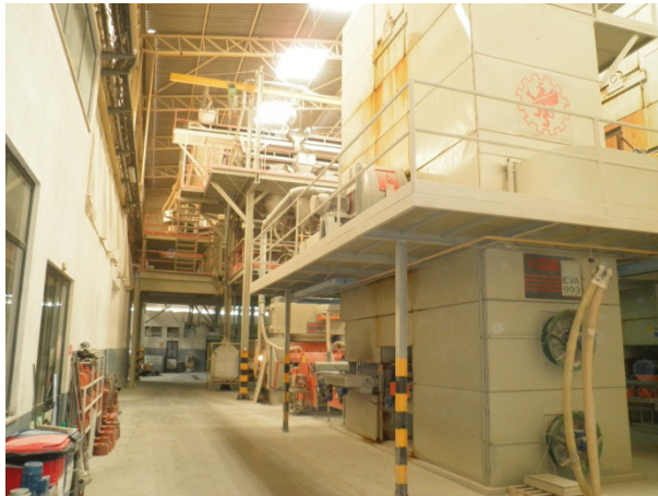
Vertical Dryer: raw tiles are dried to ~3% humidity Horizontal Multi Layer Dryer
