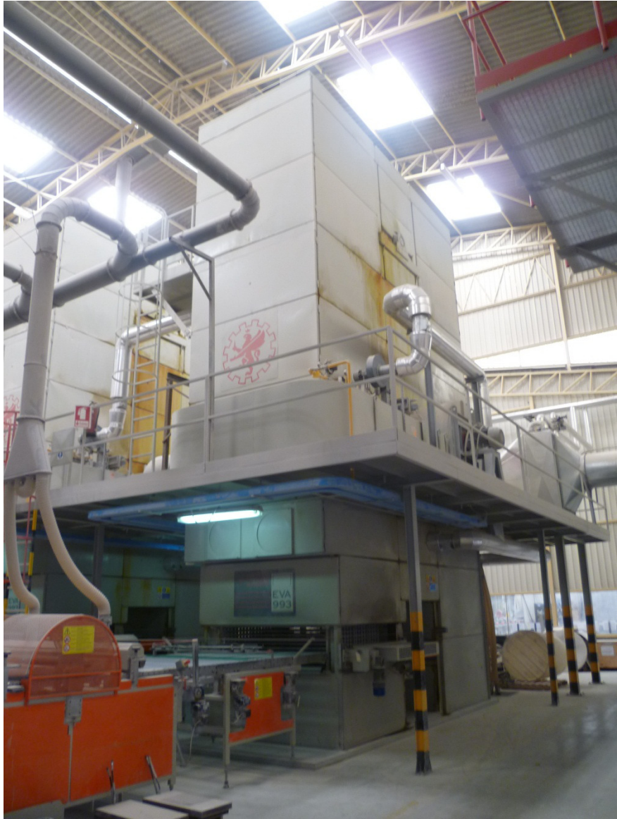
Vertical Dryers: Hot air distribution
