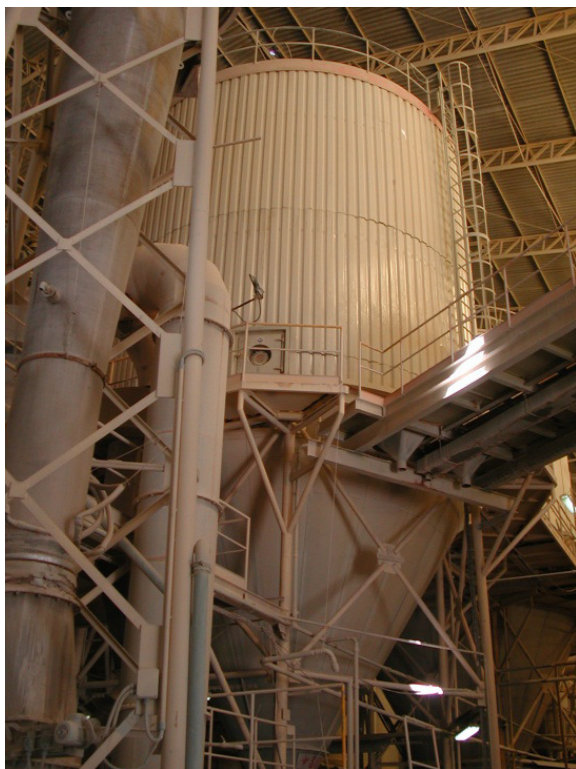
Spray Dryer: Gas heated air, 500°C, cyclone injected slur, water evaporates
