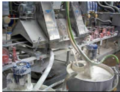
Colouring and glazing line: Moistening, Binder, Colour, Print/Molding, Decoration
