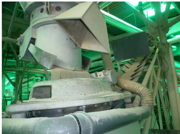
Spray Dryer: output = homogenized granulate
