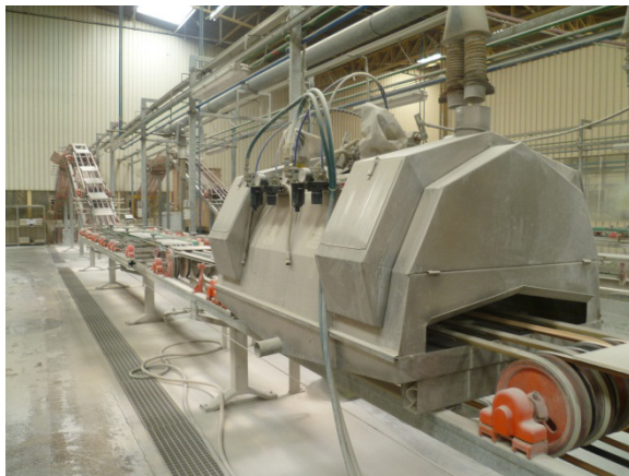
Colouring and glazing line: Moistening, Binder, Colour, Print/Molding, Decoration
