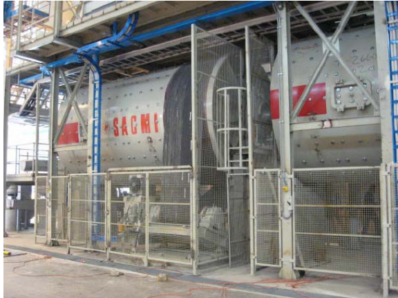
Drum mill: milling and mixing raw material
