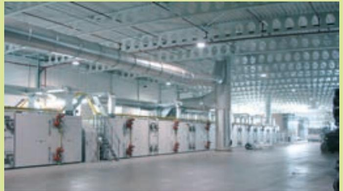
1. Inverter-controlled circulating air fans for adjustment of the air circulation intensity above and below
