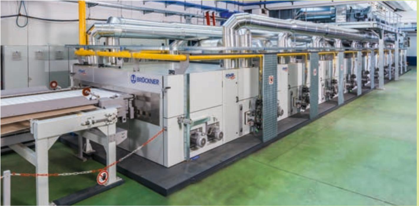
A distinguished feature of the BRÜCKNER universal dryer is the variably adjustable distribution of air and an extremely uniform distribution of temperature. The dryer is fitted with various types of fabric transportation and heating systems, depending on the process and areas of application.
