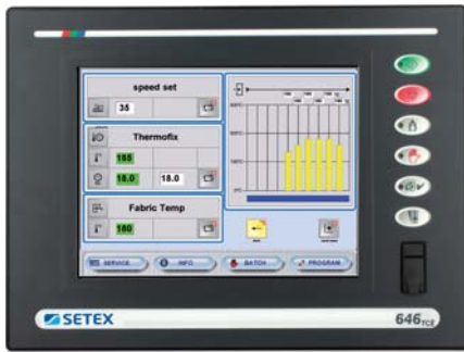
► HeatSET Control: The display shows the actual temperature profile and the preset dwell time.
